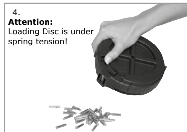
Release the loading disc slowly by stopping with your thumb.
